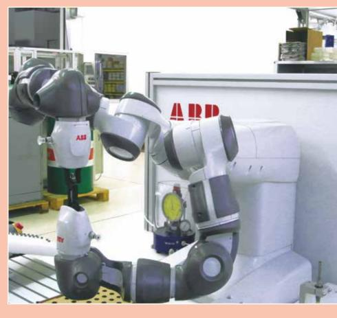
second component from the corresponding tray; then, the valve, which has already been tested, is assembled, as the robot is capable to move in space moving back to the same spot with an accuracy of 0.02 mm.
